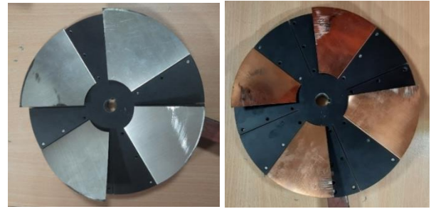
Fig. 13. Photographs of post-tested FTB with 60° steel and 45° copper foils.
