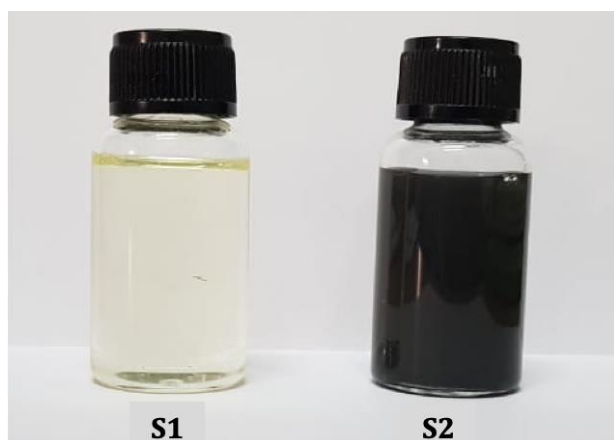
Fig. 1. Lubricant specimens: S1 (palm methyl ester), S2 (palm methyl ester + graphene).
