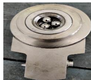
Fig. 3. Orientation of chromium coated steel balls.
