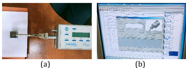
Fig. 9. The SURTRONIC 3+ type profilometer - the measurement process: a. measurement process; b. image on the monitor.
