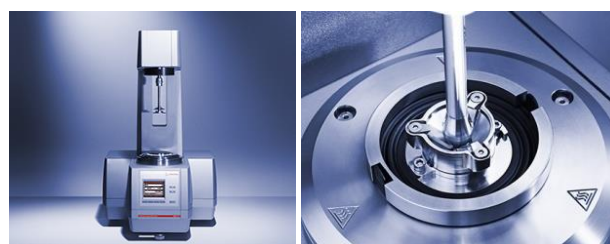
Fig. 2. The rotational rheometer MCR 102 with tribological cell T-PTD 200 [55].
