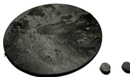
Fig. 1. Pins cut from Injection moulded discs.
