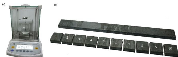
Fig. 2. (a) Densometer (b) Samples for density and hardness test.
