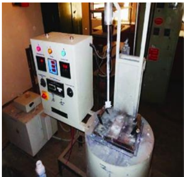
Fig. 2. Stir casting Furnace with electric heater.
