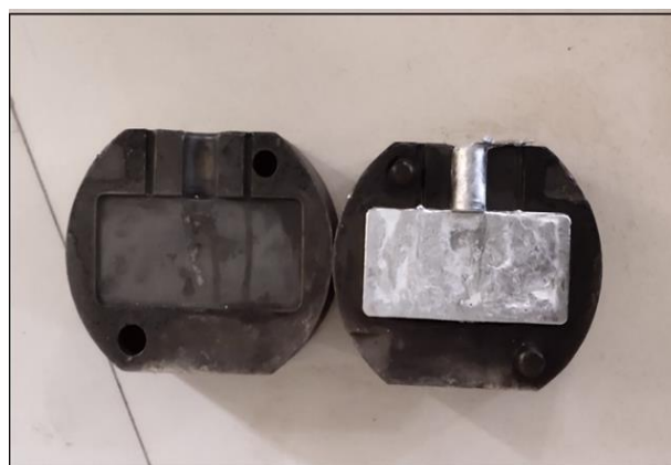
Fig. 1. Photograph of fabricated hybrid composite with die.
