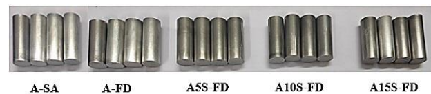
Fig. 2. The sintered composite samples.
