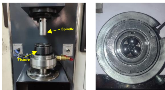
Fig. 2. Four ball fixture and spindle configuration.
