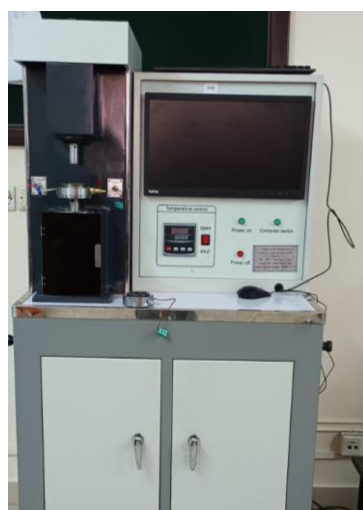
Fig. 1. Vertical universal friction testing machine (MMW1A).
