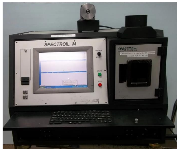
Fig. 3. Rotating Disc Electrode Optical Emission Spectrometer.
