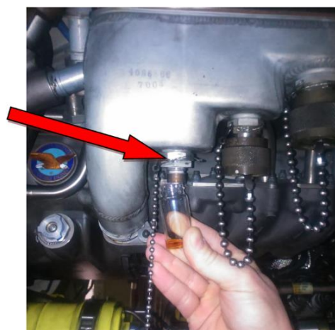
Fig. 4. Engine oil tank sample port.
