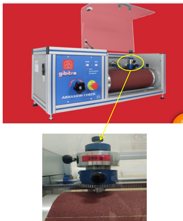
Fig. 2. (a) Abrasion Check tester gibitre instrutment, (b) The device used in the wear and abrasion tests Showing sample -counter (abrasive emery paper with #60 grit size) (254 microns).
