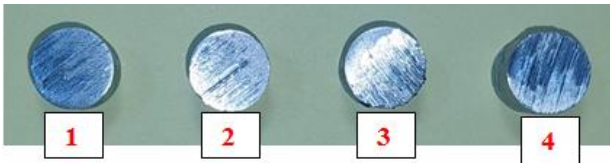
Fig. 15. Macrographs of worn surfaces for samples (1,2,3,&4) as summarized in Table 3.
