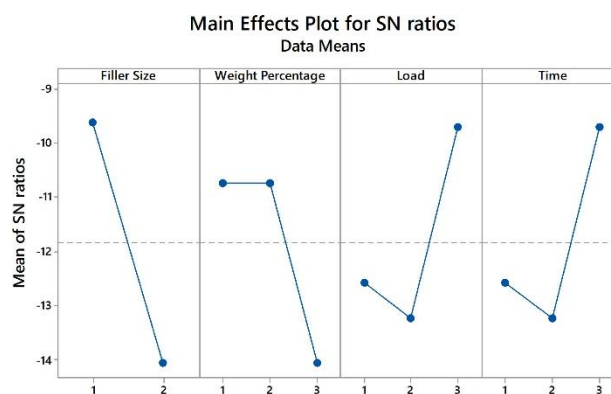
Fig. 2. Signal to noise ratio of various factors and their levels.
