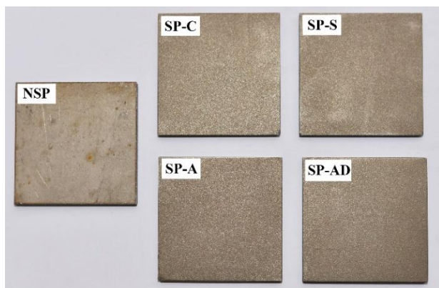
Fig. 1. Photographs of prepared flat specimens for testing: the NSP specimen is unprocessed, while SP-C, SP-S, SP-A, and SP-AD specimens have been treated with respective shot peening methods. Note the visual differences in surface appearance due to varying peening intensities and sequences.
