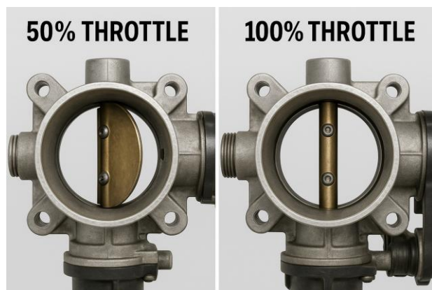
Fig. 5. Throttle percentage and butterfly.
