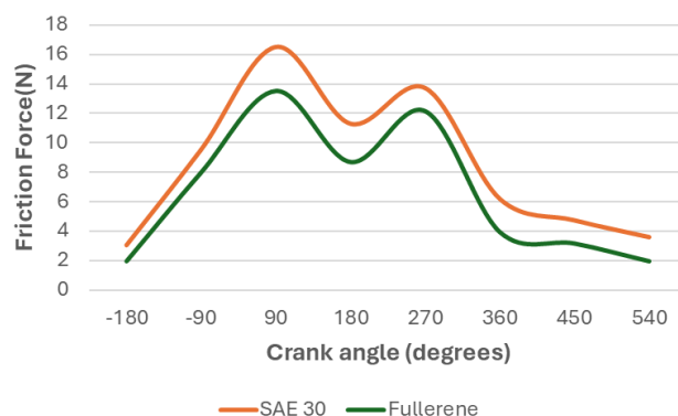
Fig. 31. Viscous friction of lubricant SAE 30 and the lubricant containing fullerenes at 1500 rpm 100% throttle.
