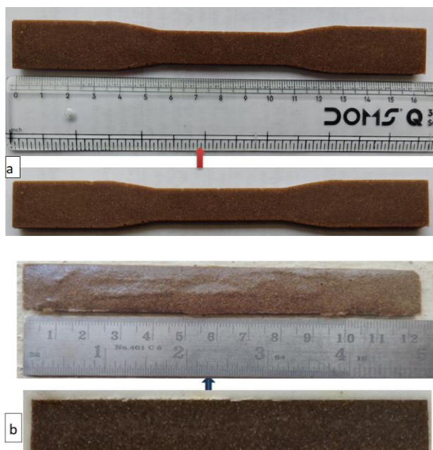
Fig. 1. (a) Tensile test specimens as per ASTM D638, (b) flexural test specimens as per ASTM D790.
