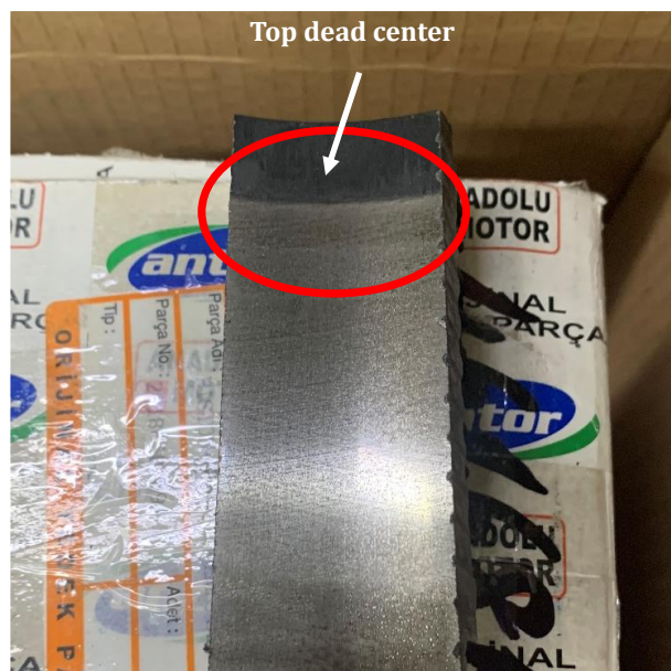
Fig. 10. Top Dead Center region of the cut cylinder sleeve.
