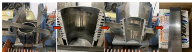
Fig. 9. At the end of the engine tests, the cylinder sleeves were cut on the metal cutting device without damaging the surface.
