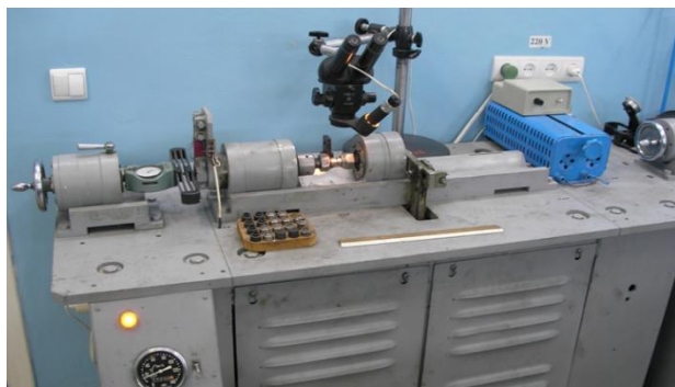
Fig. 1. Appearance of the MFK-1 machine for testing the wear of structural materials during fretting.
