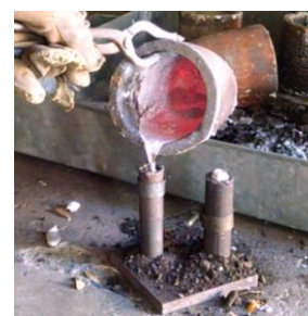
Pouring Molten MMC's in Moulds
