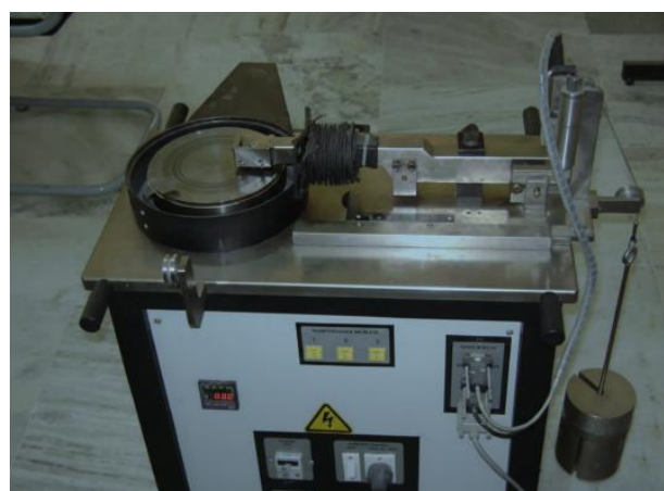
Fig. 8. Pin on disk setup.
