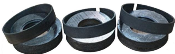
Fig. 5. Coating separated from the base steel
