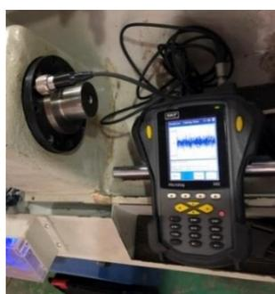
**Fig. 2.** The experimental apparatus; 1. Pneumatic cylinder generates a radial force; 2. Pneumatic cylinder generates an axial force; 3. Indicator; 4. Vibration sensor; 5. Spindle bearing; 6. The temperature controller, 7. Spindle speed controller, 8. Vibration measurement and analysis equipment, 9. Pneumatic cooling lines.
