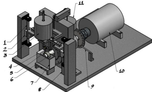
**Fig. 4.** Block and disk test setup
