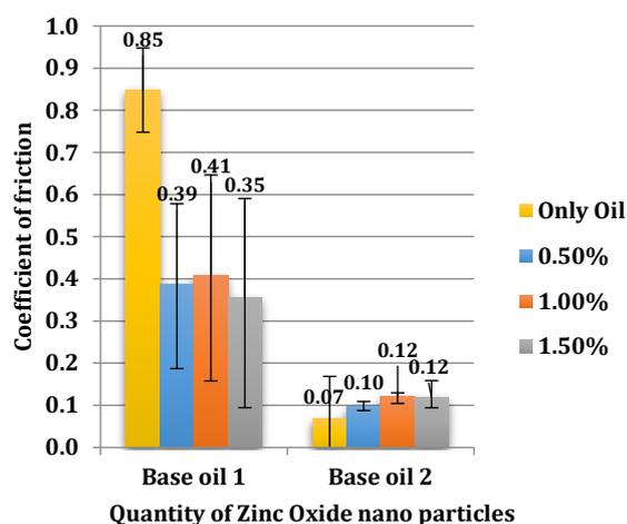
Fig. 7. Experimental results of Coefficient of friction for two base oils
