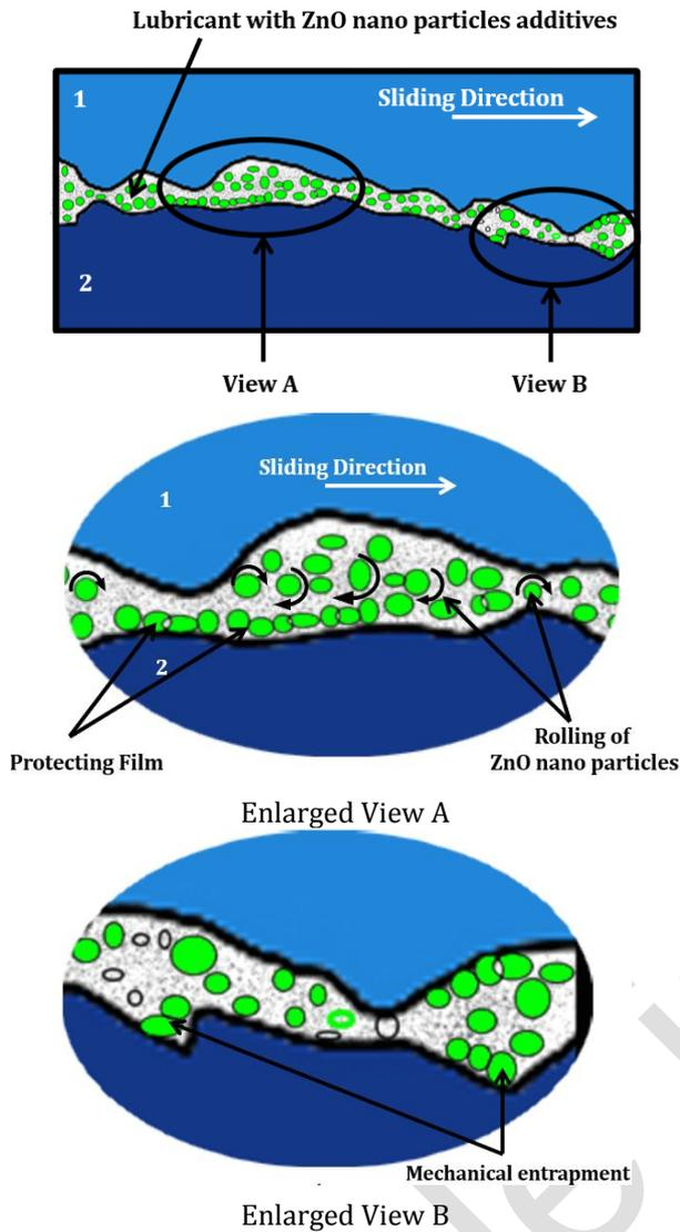
**Fig. 3.** Types of mechanisms: protective film, rolling & entrapment.
