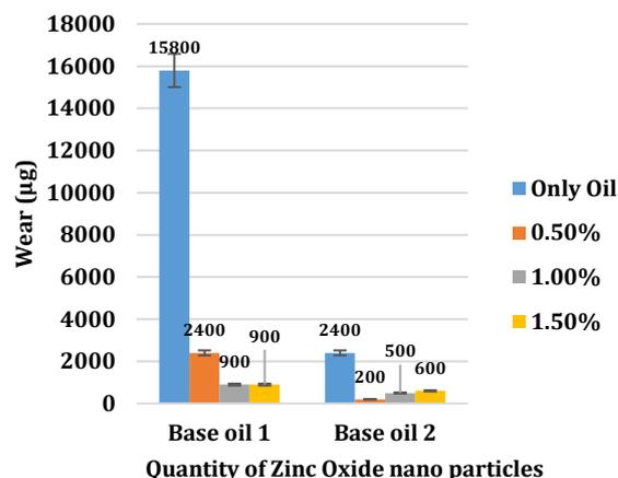
Fig. 8. Effect of base oil on Wear of blocks with Zn Oxide nano particles additive
