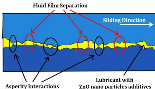
Fig. 2. Mixed lubrication conditions.
