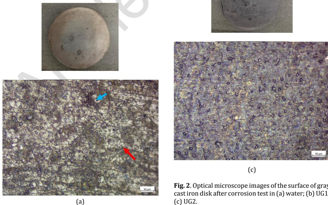
**Fig. 2.** Optical microscope images of the surface of gray cast iron disk after corrosion test in (a) water; (b) UG1; (c) UG2.
