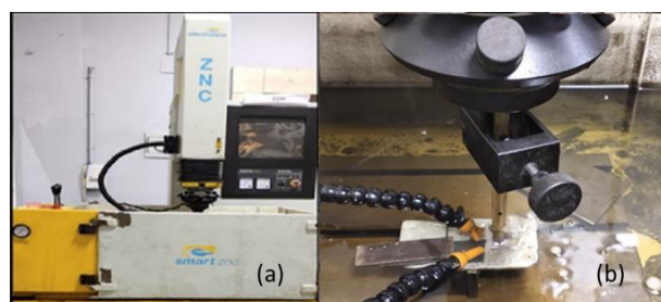
Fig. 4. Photograph showing (a) EDM machine; (b) Impressions being created during EDM.
