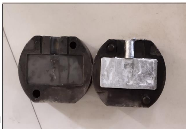
Fig. 1. Photograph of fabricated hybrid composite with die.
