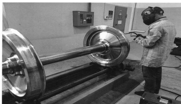
Fig. 4. Wheel Quenching with Wheelset Rotation.
