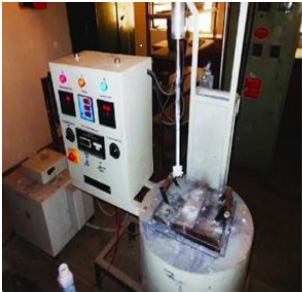
Fig. 2. Stir casting Furnace with electric heater.
