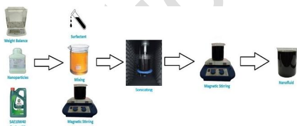
Fig. 6. Two-step method preparation of nanolubricant.
