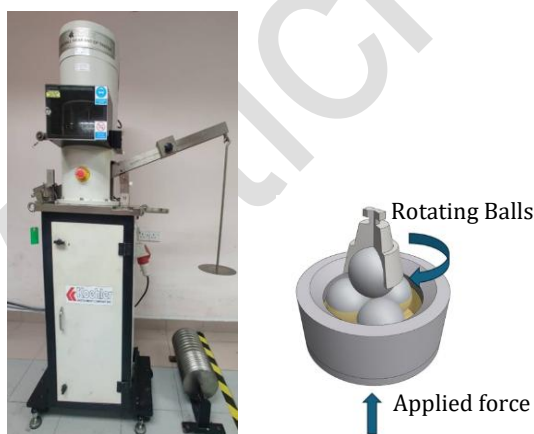
Fig. 3. Schematic diagram of the four-ball operation.
