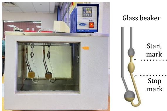
Fig. 2. Schematic diagram of a viscometer.
