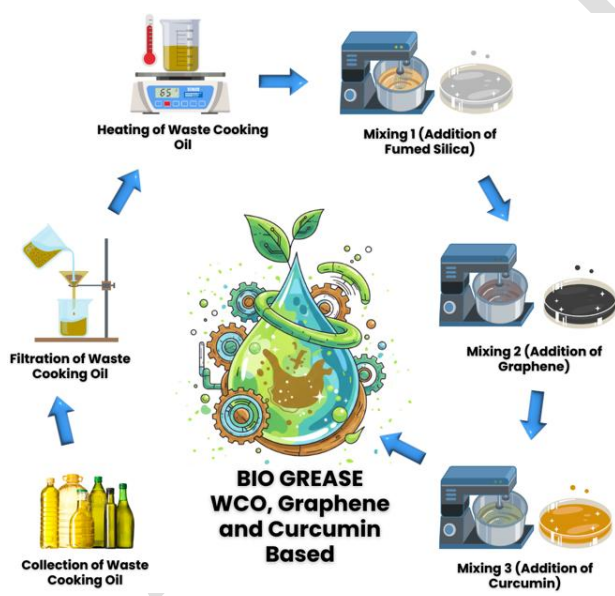
Fig. 1. Schematic of graphene-curcumin WCO biogrease preparation.
