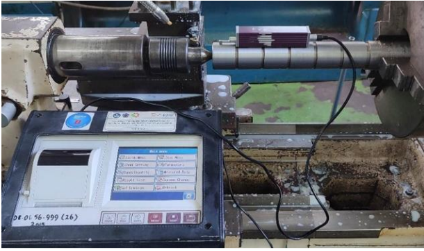
Fig. 2. Experimental setup for surface roughness measurement using a Mitutoyo SJ-410 portable surface roughness tester.
