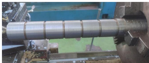
Fig. 1. Segmented AISI 1045 steel workpiece showing circumferential grooves used to separate the machined sections for surface roughness measurement.
