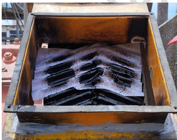
Fig. 8. Spray pattern of the lubricant in the gear.
