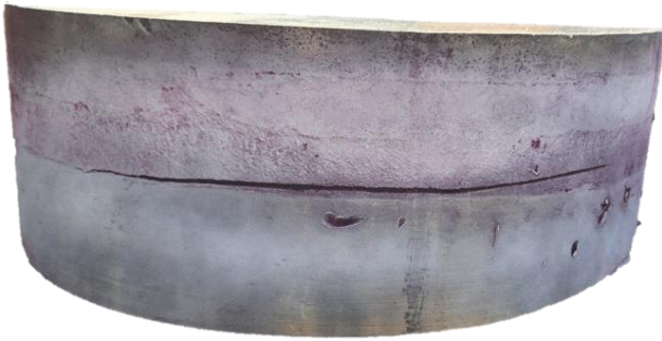
Fig. 6. Conveyor pulley shaft examined with liquid penetrant test.
